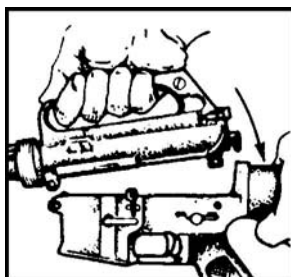
Figure 35. Joining the upper and lower receivers.
